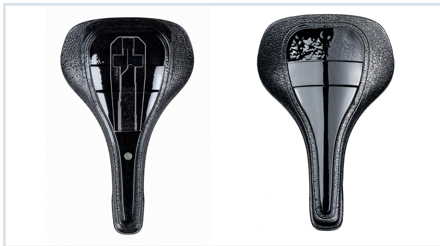
Fig. 7. EPP saddle as a technology demonstrator: functionalized with a printed circuit and flow-coated with clear coat to investigate the depth effect (left); flow coated with "piano black" PU (right) in different layer thicknesses (0.5 mm, 1.5 mm and 2.5 mm), in order to illustrate the color intensity (© ThiM-Netzwerk)
