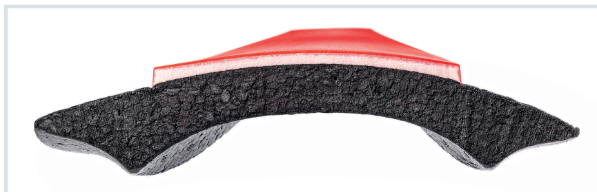
Fig. 6. After pretreatment with plasma, EPP can be flow-coated with a semi-rigid foam, with which this pattern is flow-coated with a further PU system (© ThiM-Netzwerk)
